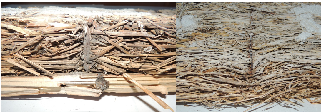
Fig. 1. Strawboard panel Solomit : left – cross-section of material attached to wooden structure; right – material stitched with steel staples
